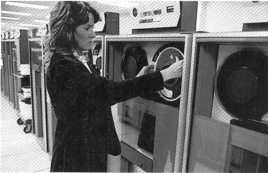
Fig. 3.14: Mounting of Magnetic Tape on Drive
